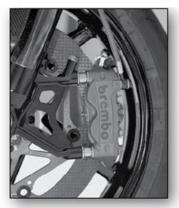
monobloc (with titanium pistons) and the whole bike weighs but 295 pounds "with a splash of gas" in the stock. Hypermotard fuel tank, you don't really need the extra unsprung mass of the second brake. "Why do I need two front brakes when the bike is so light? When he rides this, it'll be 40 minutes at a time with the front wheel up in the air."
