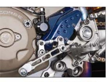
Shark-like teeth on the titanium footpegs will hopefully keep your feet from slipping. Fine finishes abound on the Leggera.
