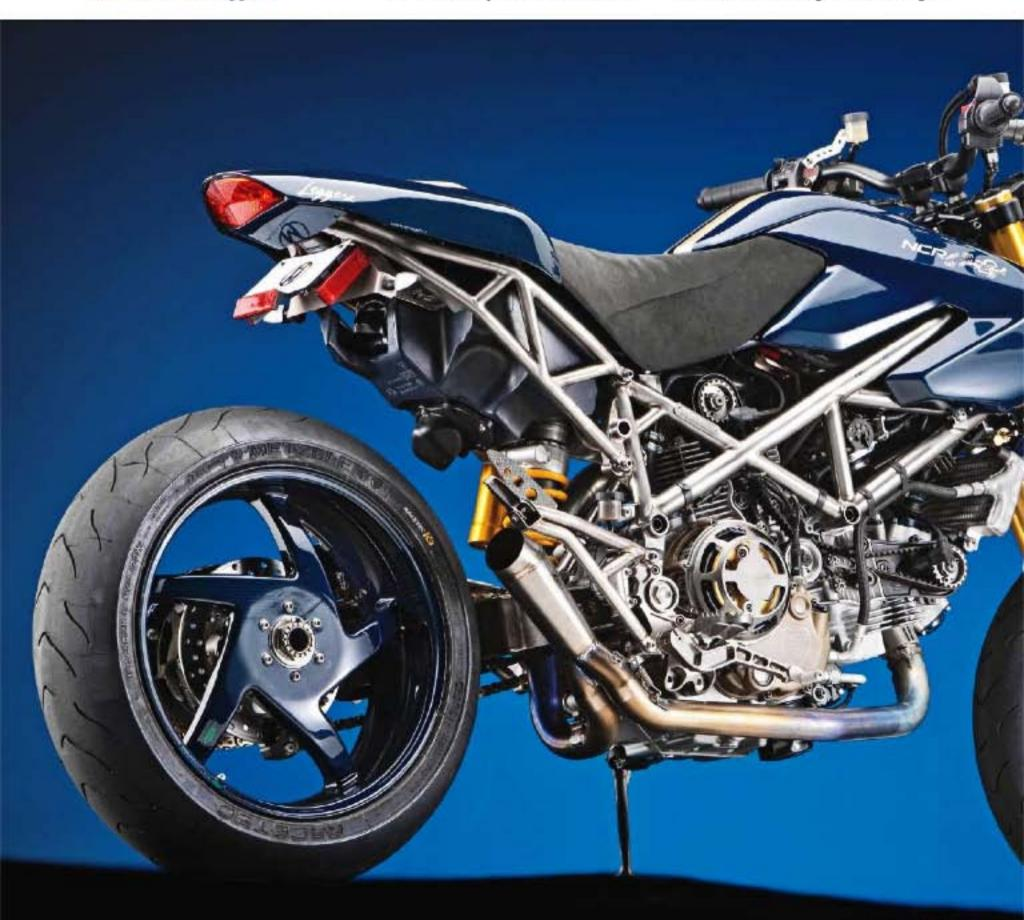
Öhlins 46mm fork with Ti-nitride coating and NCR Corse billet bottoms are held by NCR tripleclamps made from "avionic" aluminum. Öhlins shock features NCR Corse valving.
