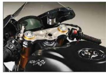
the latest, top-line Öhlins GP suspenders, tuned in-house by NCR Corse. An FGR000 43mm inverted fork (carried in adjustable-offset triple clamps) and a TTX ride-height adjustable shock carry this oh-so-light load. Brembo Monobloc brake calipers work on ultra-light Brake Tech Axis ceramic-composite discs.
