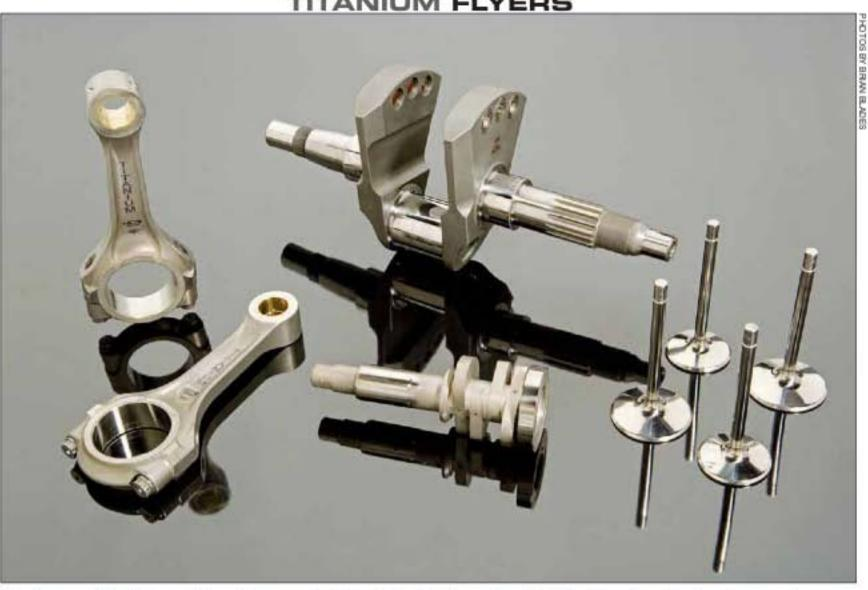
Stroker crankshaft is machined from a giant steel billet. "Dimensionally, this piece is not going to move," says NCR's Joe Ippoliti. It costs \$6600 and is made by the same people who make F-1 car racing crankshafts. Performance cams are \$627 apiece, while the Ti valve kit is \$1400. Ti rods, machined from a forged billet for 8 hours, cost \$3800.
