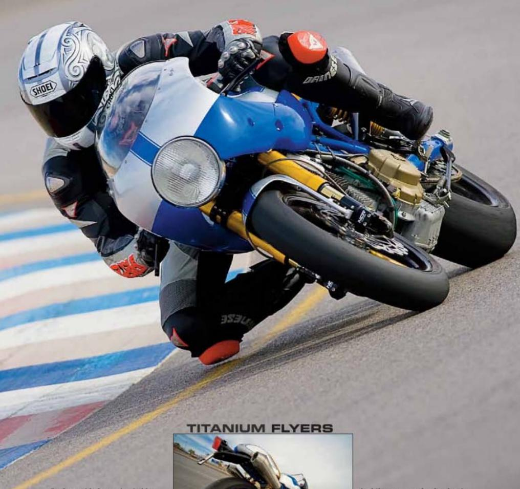
Such as with the engine in New Blue, a step up the seriousness ladder if only because this bike had one of NCR's lighter and more powerful two-valve Desmo engines displacing 1078cc. This was the so-called One Shot engine, with all the lightweight internals, billet crank, etc.
