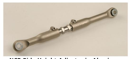
NCR Ride Height Adjustor in Aluminum High quality ride height adjustor in aluminum. Weight: 276 gm.
