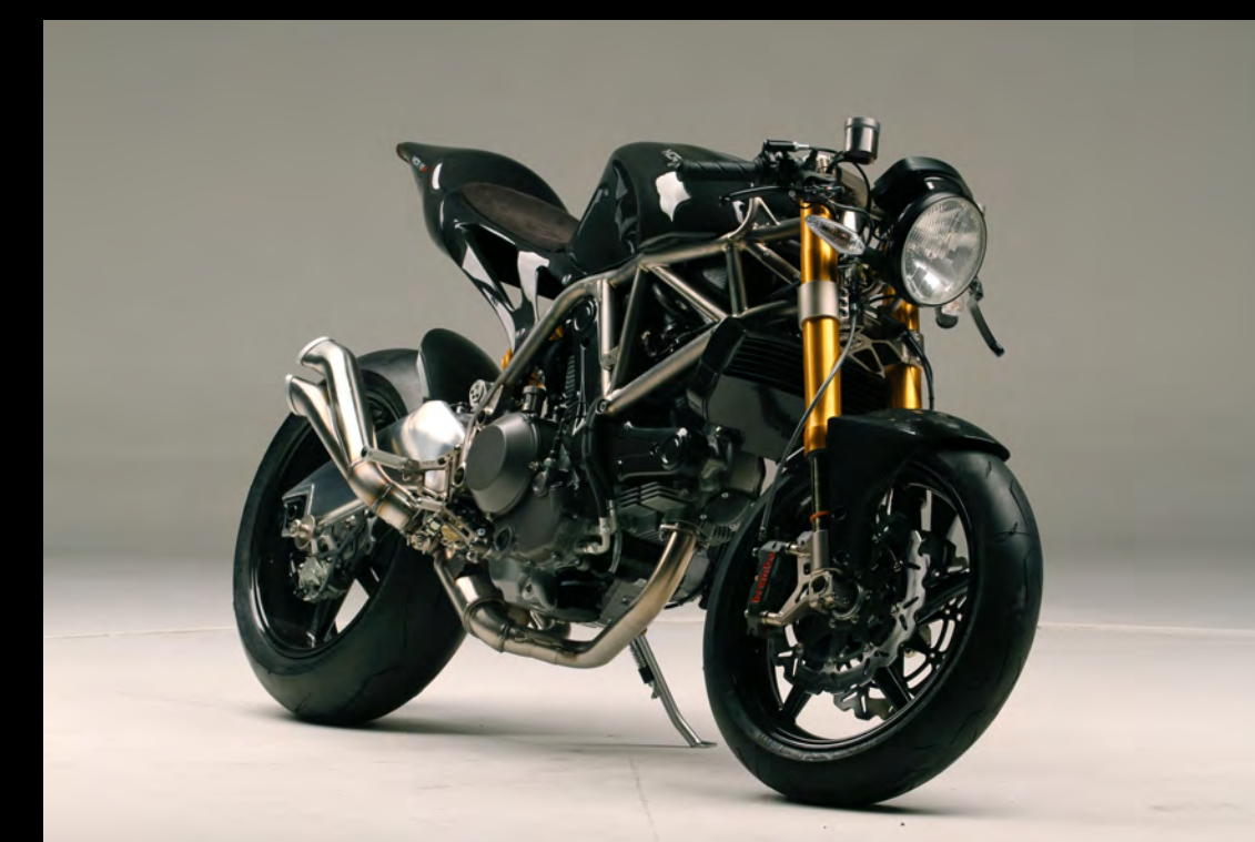
NCR M4 and NCR M4 One Shot The new standard in performance. Titanium frame, carbon everything else. Being homologated for the street. 302 lbs and 296 lbs with oil and battery. No Longer Available
